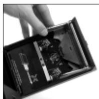
2 Place your thumb on the edge of roller unit and turn the unit up and take out the roller.
