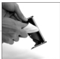
3 Clean the roller with a lens free cloth dampened with water.
