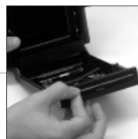
5 Check the film exit debris. Remove paper or dried reagent from the film exit.
