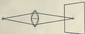
Fig. 18. Rays Bent by Double Prism.
