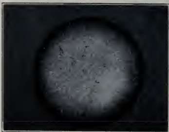
Fig. 40. Spot on Gelatine Caused by Moisture.
